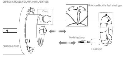
pull out the protective grating, pull the modeling lamps straight out of the sockets. Insert the new modeling lamps straight into the sockets. Push the protective grating in to place. Secure with the
